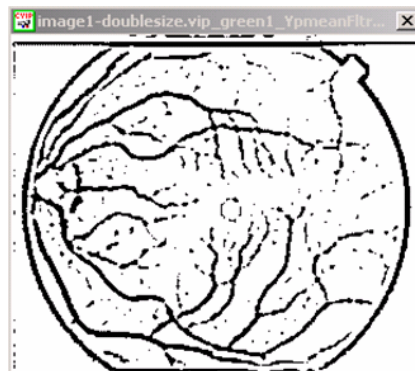
Fig 21. Algorithm 2: Post processing step 3. Grayscale-to-binary conversion: The gray scale image was converted to binary by using a binary threshold.
