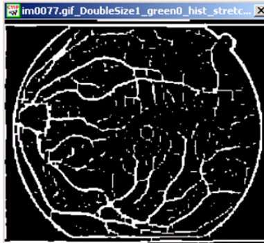
Fig 11. Post processing step 3: Logical NOT operation & Hough Transform. The NOT operation produced a black background. The Hough transform was used to attempt reintegration of bifurcation points and vascular branches
