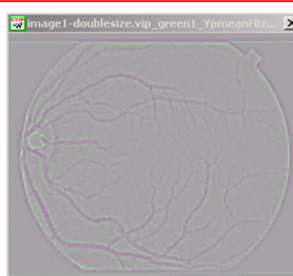
Fig 18: Algorithm 2: Edge detection. Edges of the Y_p -mean filter-filtered image were detected using a Laplacian edge detector to segment blood vessels out of the image.
