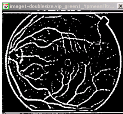
Fig 22. Logical NOT operation & edge linking. The NOT operation produced a black background with white objects. Edge linking was used to attempt reintegration of bifurcation points and vascular branches.
