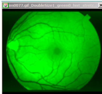
Fig 5. Preprocessing step 2: A histogram stretch of the green band image helped enhance contrast.
