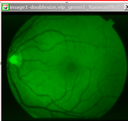
Fig 17. Algorithm 2: Preprocessing step 2. The Y_p mean filter eliminated noise from the green band and produced a smoothing effect.
