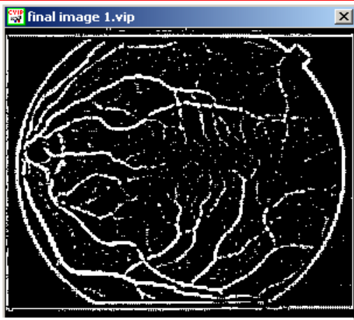
Fig 28. : Blood Vessel Segmentation Algorithm 2's output image A. Degree of match to hand-drawn image using: Pratt's figure of Merit: 0.6685 Signal to Noise ratio: 10.536 Root mean square error: 65.810
