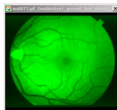
Fig 6. Morphological filtering operation. An opening operation with a size-5 rectangular structuring element smoothed the vessels' geometries.
